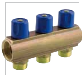
Collettore da barra con attacchi maschio 3/4 Eurocono, valvole incorporate, interasse 50mm Manifold made of brass rod with 3/4 Euroconus male offtakes and incorporated valves, interaxis 50mm Colector de barra con empalmes macho Eurocono 3/4, válvulas incorporadas, distancia entre ejes 50mm
