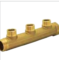
Collettore a 3 attacchi filetto maschio 1/2", interasse 50mm Manifold with 3 male offtakes 1/2", interaxis 50mm Colector de 3 empalmes rosca macho 1/2", distancia entre ejes 50mm
