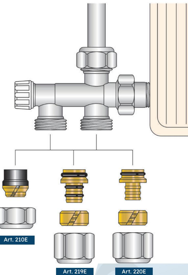
Valvole monotubo e bitubo | Monotube and bitube valves
