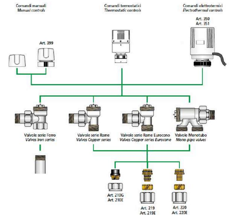
Valvole termostatiche serie THERMO | THERMO thermostatic valves
